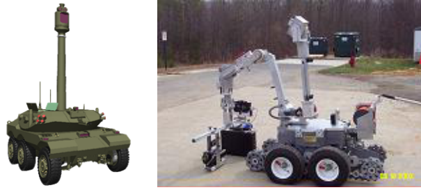
Figure 19. Left: Example of a mast mounted (16 ft high) EO system for ARV in the US FCS program. Right: The RONS with a manipulator arm for remote ordnance neutralization.
