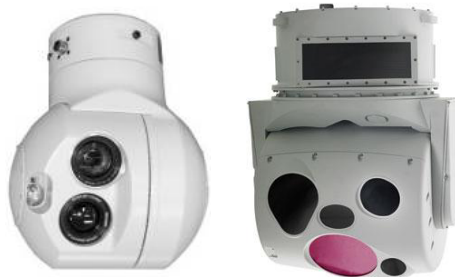
Figure 20. Two examples of sensor gimbals. Left: DST Colibri DUO gimbal with IR and TV cameras and a laser range finder, weight 1.7 kg. Right: ASTAMIDS gimbal employing an integrated, EO infrared/multi-spectral imaging payload, including an illuminating laser and a laser rangefinder/designator. The sensors can detect obstacles, combat vehicles, and other targets, including those under camouflage.
