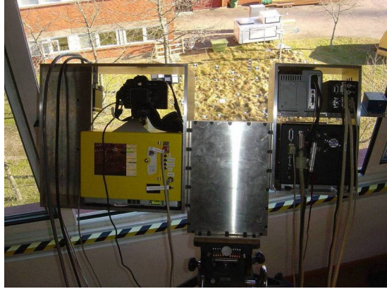
Figure 3. The sensors mounted on a tripod, looking through at the grass test area outside the roof-top lab at FOI.
