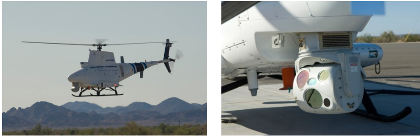
Figure 18: The Northrop Grumman Fire Scout unmanned helicopter carrying the ASTAMID's sensor package for land mine detection. It includes a multispectral EO/IR sensor, a laser illuminator and a laser designator.
