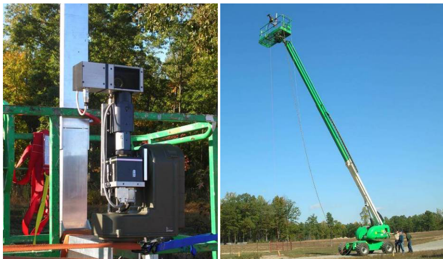
Figure 4. During participation in the NATO SCI-193 pilot test at Fort A.P. Hill, the hyper-spectral imager Imspec was mounted on an elevated platform (left) on a cherry picker (right).
