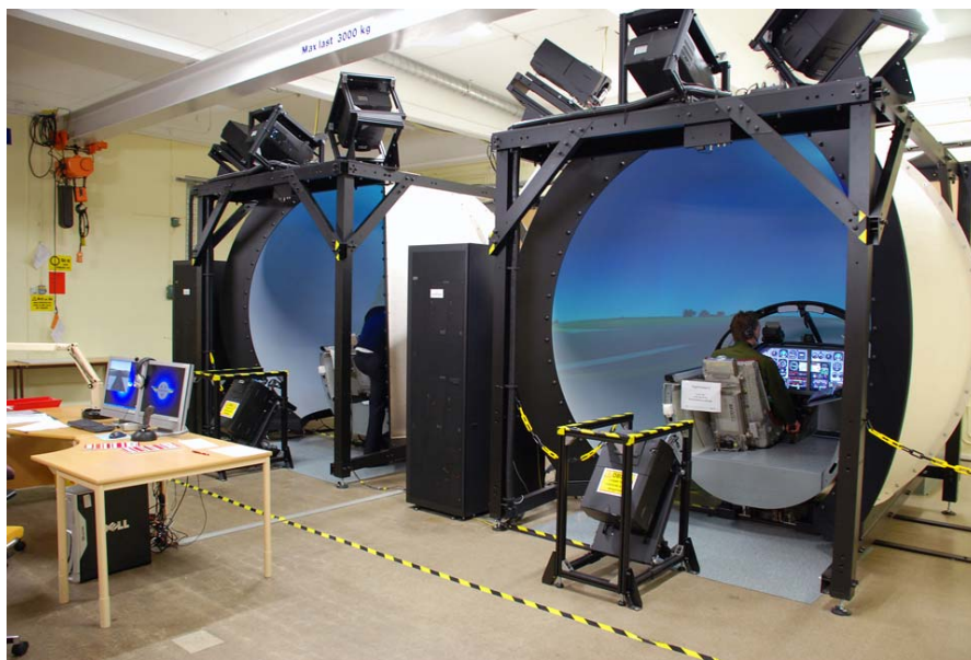
Figure 12. The two pilot stations in Flightbook. From the control station, at the table behind, a third person can act as air-traffic controller or air supreme commander.
