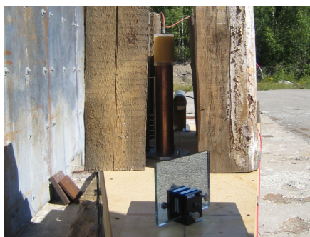
Fig. 6. Photo of experimental set-up showing the argon flash bomb located behind the HE-filled copper cylinder.
