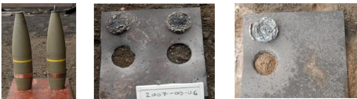
Figure 1. Donor and acceptor 15 cm apart (left). Witness plate with two detonations of acceptor consisting of TNT (middle). Witness plate with no detonation of acceptor consisting of GUNTOL (right)
