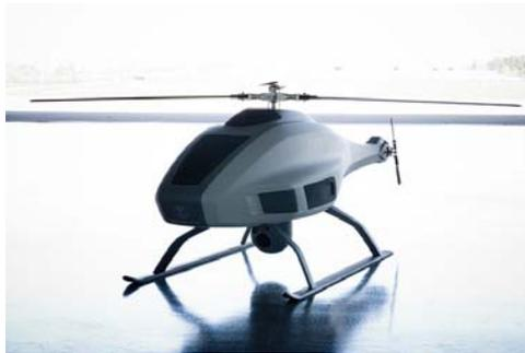
Figure 5. The UAV helicopter Skeldar from Saab Aerosystems.
