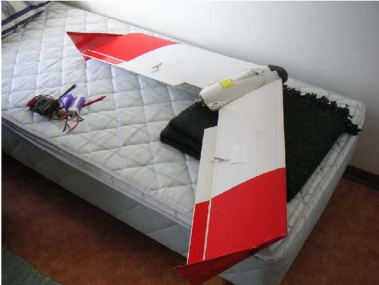
Figure 8. The small UAV SmartOne by SmartPlanes (<http://www.smartplanes.se/>). The photo is taken at the occasion for a survey of shallow bottoms in the Interregional project ULTRA ([http://www.kvarken.fi/Pa\\_svenska/Projekt/Ultra](http://www.kvarken.fi/Pa_svenska/Projekt/Ultra)).
