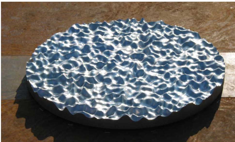
Figure 5. The rough aluminium surface. The diameter is 0.9 meter.
