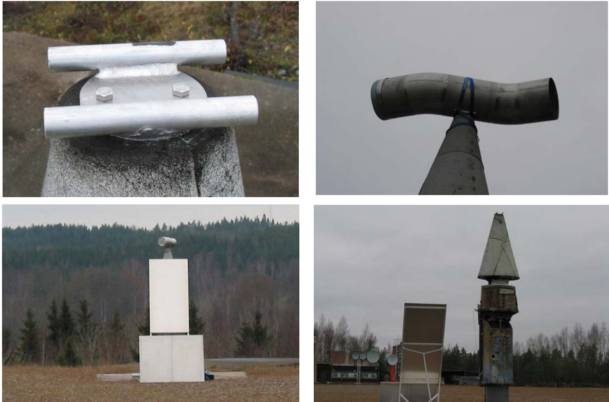
Figure 7. The upper left picture shows the support that is attached to the turntable. The upper right picture shows the cavity placed on the support and how the cavity is tied with a band to the support. The lower left picture shows a view of the setup from the antennas. The lower right picture shows the setup from behind the pylon. The two parabolic antennas that have been used can be seen between the ladder in the background.
