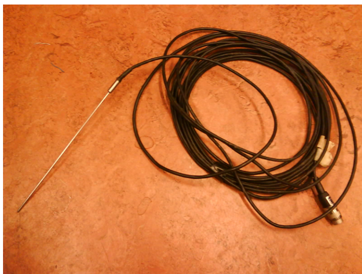
Figure 6-3. The figure shows one of the 24 Pt-100 resistance thermometers
