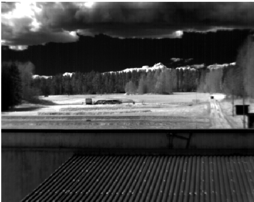
Figure 3-10. Image taken with Cheetah-640CL with a high pass filter > 1.36 \mu\text{m}
