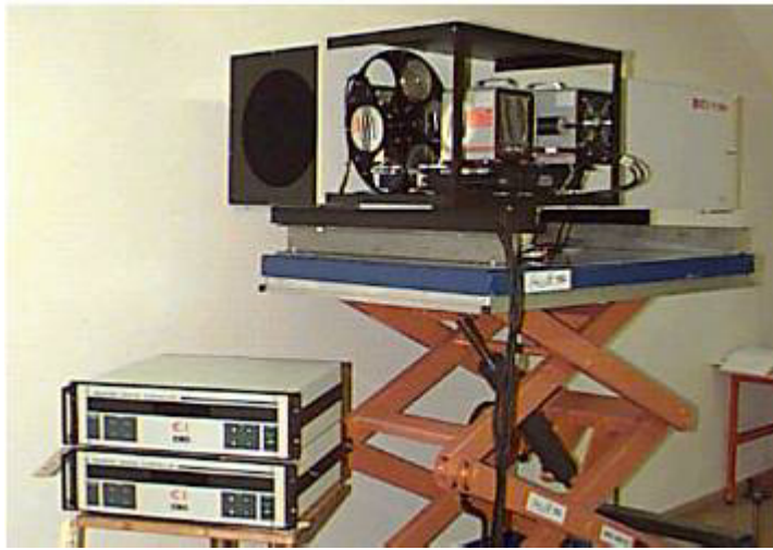
Figure 9-1. Collimator test system CTS-1; with target wheel, test targets, blackbody source and control unit.
