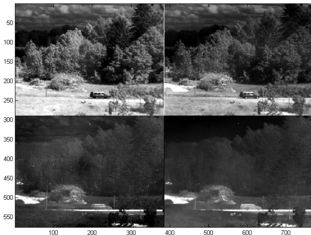
Figure 3-26. Example image: a lens with 100 mm focal length is used. Upper left: filter 1 ( 1.5 - 1.8 \mu\text{m} ); upper right: filter 2 ( 2.1 - 2.5 \mu\text{m} ); lower left: filter 3 ( 3.5 - 4.1 \mu\text{m} ); lower right: filter 4 ( 4.5 - 5.5 \mu\text{m} )
