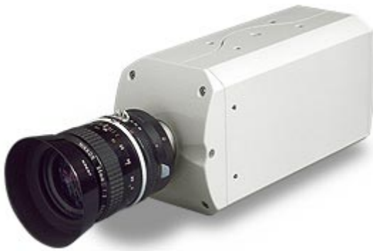
Figure 3-1. The high speed visual camera Phantom V4.1 (Vision Research, Inc.). At FOI a different lens is used than shown in this image.
