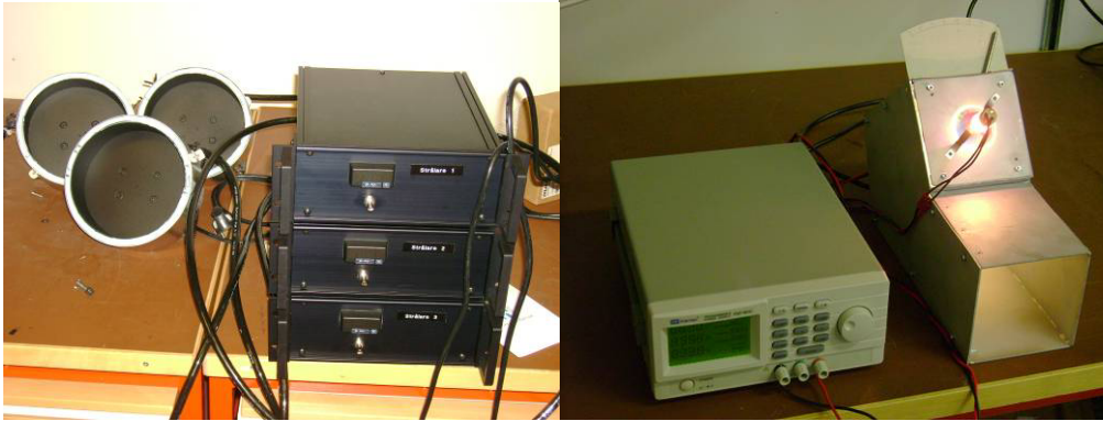
Figure 5-5. Peltier elements (left) and a lamp source (right). The temperatures of the Peltier elements are fixed and preset to 10, 25 and 50 °C. Different radiance levels from the SWIR source are obtained by changing the aperture of an iris diaphragm in front of the lamp. The lamp is driven with 12 V generating about 100 W. In the 2.1-2.5 \mu\text{m} band radiance levels between 4 – 15 \text{W}/(\text{m}^2 \cdot \text{sr}) are obtained.
