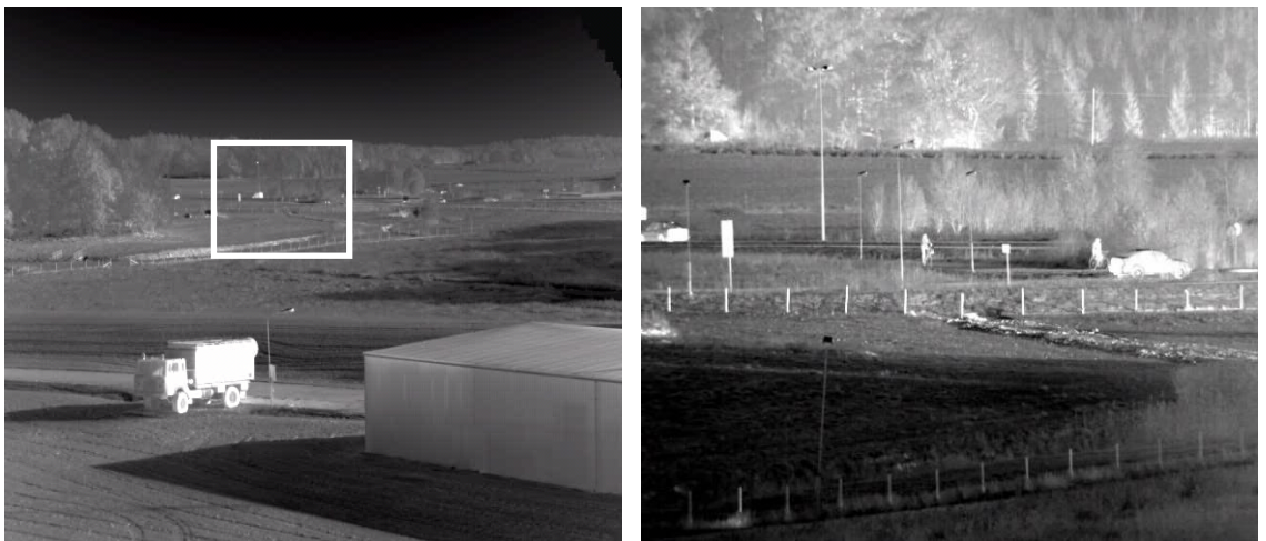
Figure 3-18. The images show two Emerald registrations in a spectral band 4.6-5.0 \mu\text{m} using two different lenses. Left: \text{FOV} = 18 \times 14^\circ , focal length = 50 mm. The white square corresponds to the right image. Right: \text{FOV} = 4 \times 3^\circ , focal length = 250 mm
