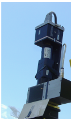
Figure 3-30. ImSpector V10E (Specim). From top to bottom: CCD array, dispersive element, scanning mirror
