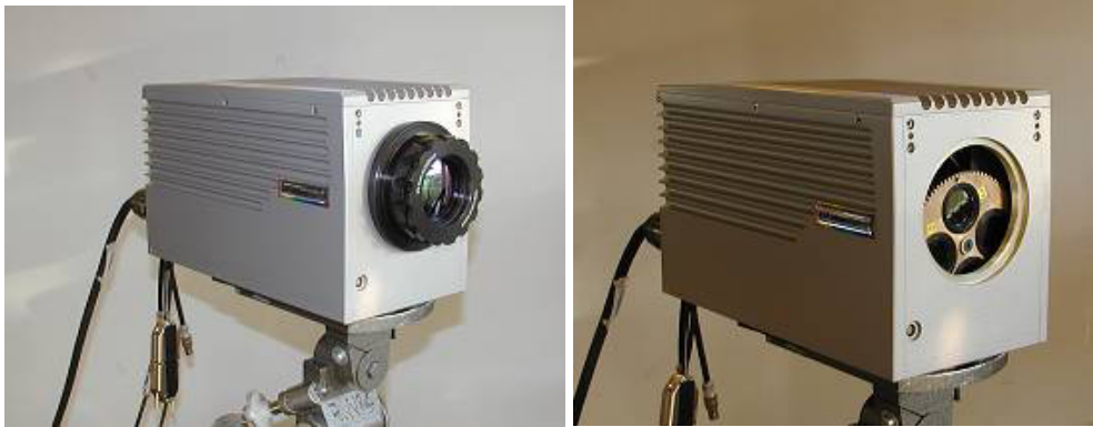
Figure 3-16. Left: Emerald with a 50 mm lens, right: Emerald with the lens removed revealing the filter holder in the middle.
