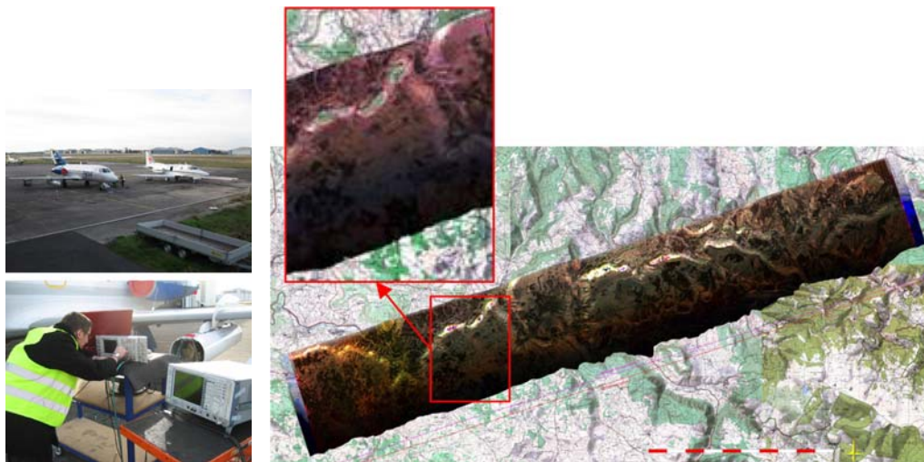
Figure 4. System calibration measurements with SETHI and LORA at Nîmes-Garons airport in preparation of the first flight mission during the campaign LORAMbis 2009 (left). Bistatic data acquired by SETHI with a bistatic elevation angle of 0^\circ ("quasi-monostatic") and formed into a SAR image which is visualized on top of a map covering the area (right). The significant topographic relief of the test site is clearly visible. Three of the four different sub-bands in the stepped-frequency waveform have in this case been processed separately instead of the fully reconstructed signal bandwidth. The colour coding based on the three sub-bands is 222-305 MHz (red), 272-355 MHz (green) and 400-460 MHz (blue).
