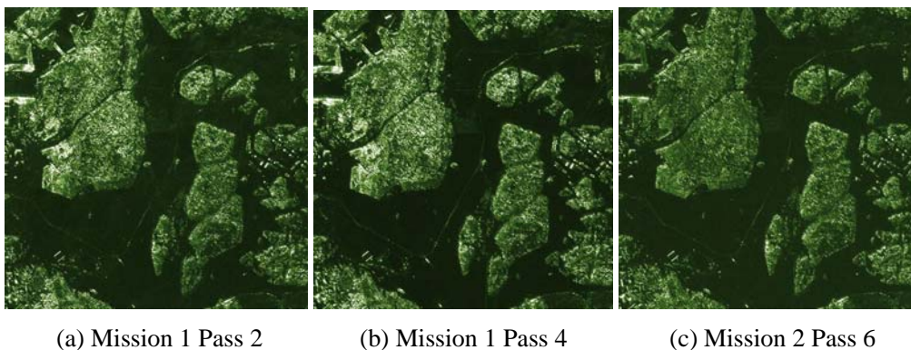
Figure 9. (a) Monostatic LORA image. (b)-(c) Bistatic image with LORA as receiver and SETHI as transmitter. Bistatic elevation angle is 0^\circ in (b) and 10^\circ in (c). Kvarn test site, flight heading 225^\circ and radar antenna is left looking. The image size is 2 km x 2 km.
