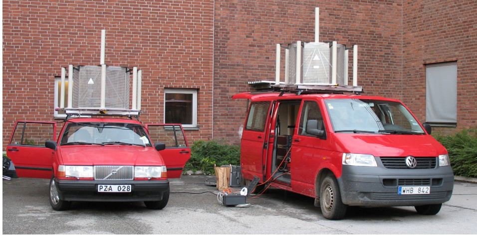
Figure 2.4: Antenna arrays mounted on transmitter (to the left) and receiver (to the right) vehicles.
