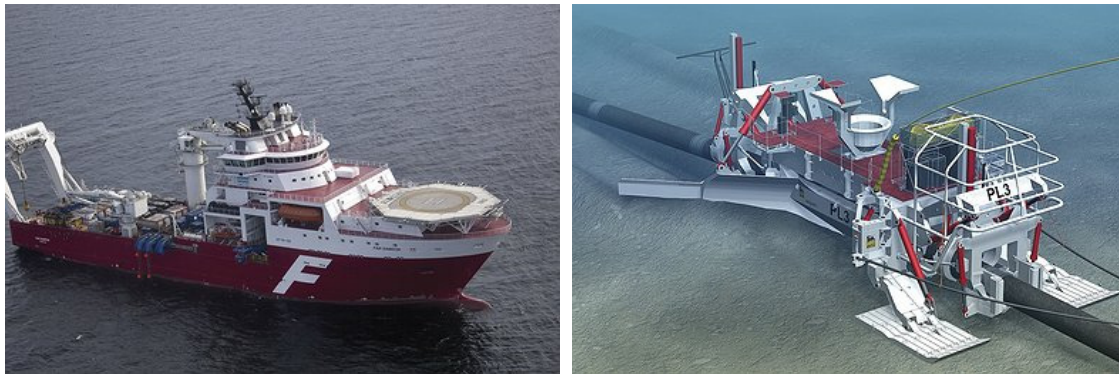
Figure 2. (a) Photo of Far Samson (post-lay trenching vessel) (b) Sketch of a plough used for post-lay trenching. (Photos: copyright of Nord Stream).
