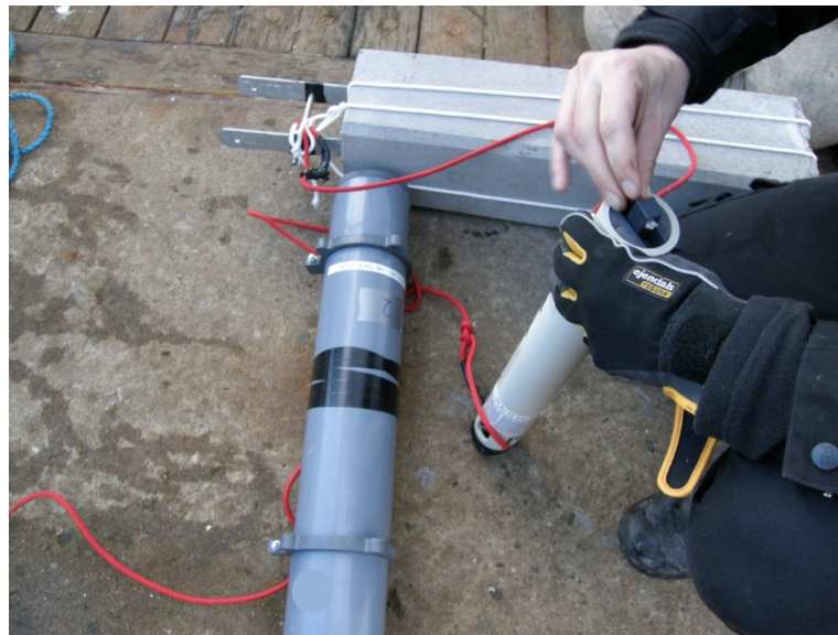
Figure 10. A rig is assembled just before deployment. Visible in the photo is the 60 kg concrete ballast weight, the dark grey autonomous DSG hydrophone system and the light grey acoustic release.
