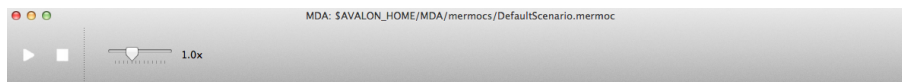
Figure 3.5: The UI toolbar has controls for starting, stopping and pausing the scenario. You can also change the realtime multiplier using the slider.
