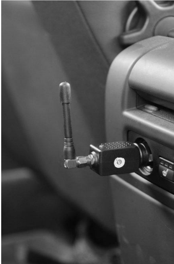
GPS jammer connected to the cigarette lighter socket in cars. (Photo: Peter Johansson, FOI)
