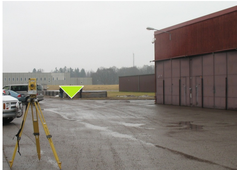
Figure 3. Photo of the total station and the starting position of each round (at the bottom peak of the triangle). The garage building is visible to the right.
