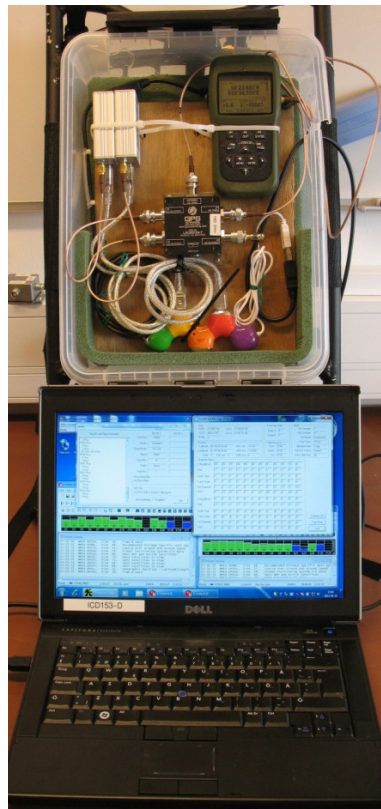
Figure 1. Two Ublox 6 GPS receivers (top left), a DAGR (top right), an antenna splitter (middle of box), USB hub (rainbow colored) connecting all receivers to a laptop.
