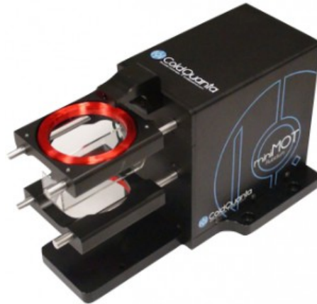
Figure 19: The mini MOT Rubidium cell from ColdQuanta [100]. This cell is already pre pumped and contains the ion pump to reach ultrahigh vacuum. With proper laser equipment and cameras a rubidium cloud can be formed with a temperature of 50 \mu K.
