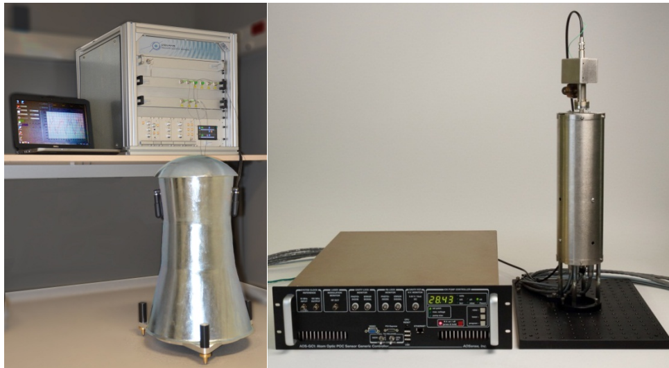
Figure 18: Left, \mu QuanS [98] commercial system that measures the absolute value of the gravity by using a cold atom interferometer [38]. Right, AOSense [99] vertical gravimeter that Lockheed Martin purchased in 2011 [37], ARW \approx 1\mu g/\sqrt{Hz} , stability < 0.1\mu g .
