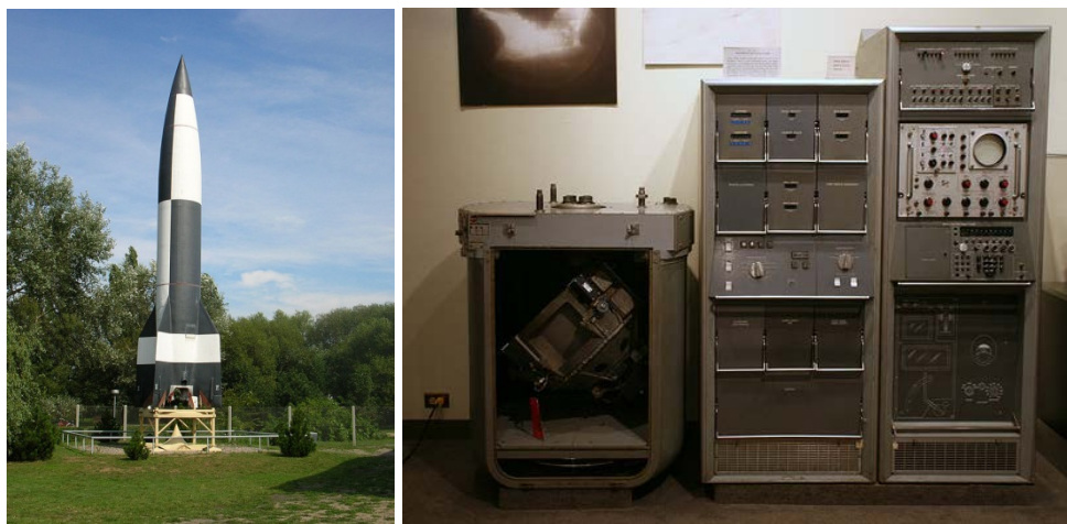
Figure 1: Left V-2 rocket which had a simple electromechanical device for inertial navigation [13]. Right, early nuclear fast attack submarine inertial navigation system, the gyroscope (left box in picture) is spinning at 20000 rpm and remains perpendicular to the axis of earth [14] because of the gimbal suspension and the law of conservation of angular momentum. Measuring the deviation of the submarine compared to the gyroscope orientation gives the submarine orientation compared to earth.
