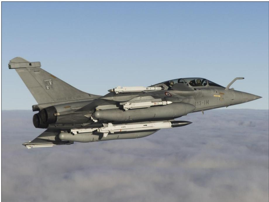
*A Rafale dual-capable fighter carrying the French nuclear armed cruise missile ASMP-A. Photo: reproduced courtesy of the French Air Force*
