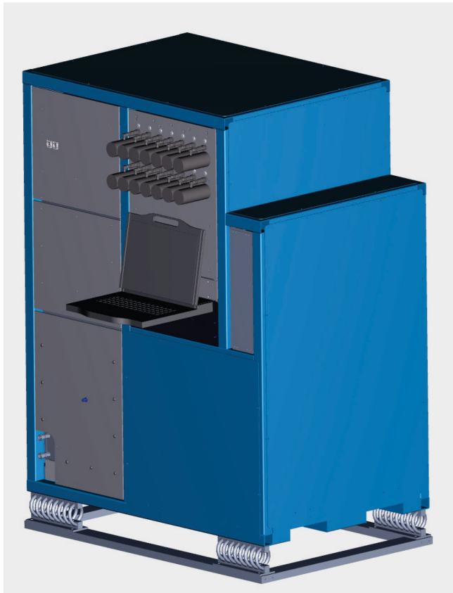
Figure 1. Overview of the new design for the SAUNA Field system. The four detectors are located at the bottom right of the system and an UPS is integrated into the custom-built frame, located above the detector units.
