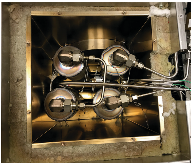
Figure 1. The sampling oven with the three new traps installed, the heating element (not shown) is located next to the wall at the bottom of the picture. The two larger traps are filled with MS4A and the smaller trap, in the centre is filled with Ag-ETS-10.
