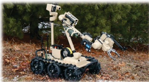
Figur 4.5: Centaur UGV. US Army Man Transportable Robotic System (MTRS) Inc II. (Foto: US Army)
