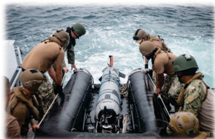
Figur 5.3: En MK18 Mod 2 Kingfish 100 (REMUS 600) tas upp i en Mark VI patrullbåt (foto: Mass Communication Specialist 2nd Class Cole C. Pielop, US Navy, public domain).
