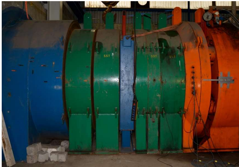
Figure 3.5 The rig is showed in the middle of the photo in the position for the air blast tests, for a wall element without the axial force applied.
