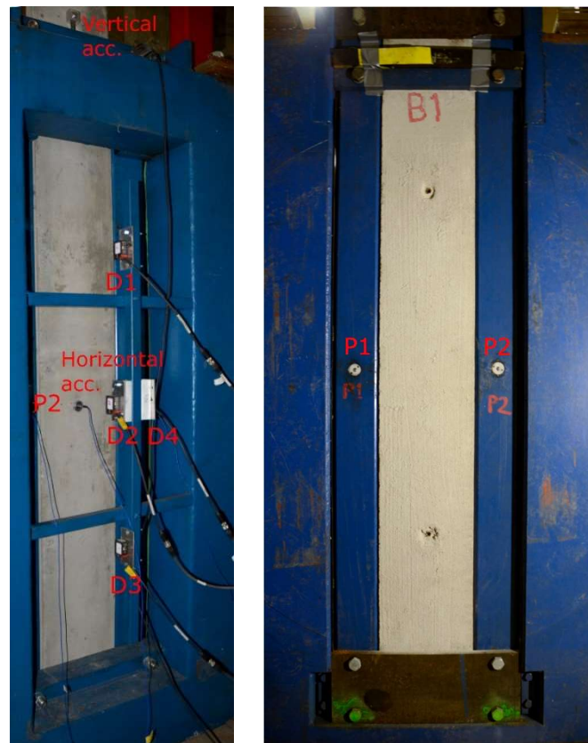
Figure 3.11 Gauge locations for displacement gauges and accelerometers shown on the backside of a wall element to the left. Locations of the pressure gauges P1 and P2 shown from the front of the wall element are shown to the right. The same locations for these measure locations were used for the previous study by Berglund and Hansson (2017), except for the vertical accelerometer that was not used for the previous study.
