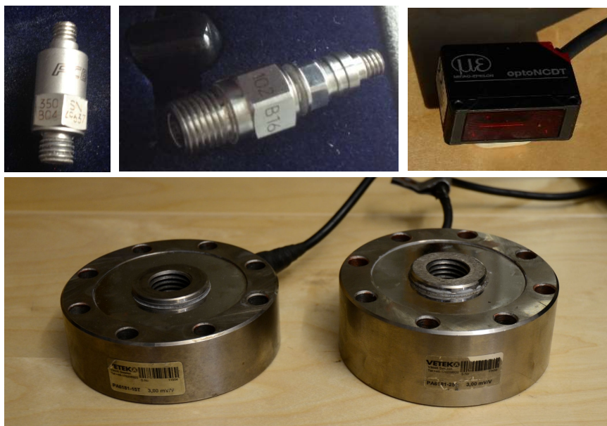
Figure 3.9 A line-up of different gauge types used for the experiments, shown top left PCB 350B04 \pm 5000 g accelerometer, top middle PCB 102B16 pressure gauge, and top right optoNCDT laser displacement gauges 1420-200. The lower photo show VETEK PA6181-15t (left) and VETEK PA6181-25t (right) force transducers.
