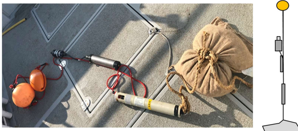
Figure 3. Photo and rig design of the hydrophone rig with a gravel bag as ballast weight, an acoustic releaser (light grey), a Soundtrap hydrophone system (black) with external battery pack and floatation buoys.
