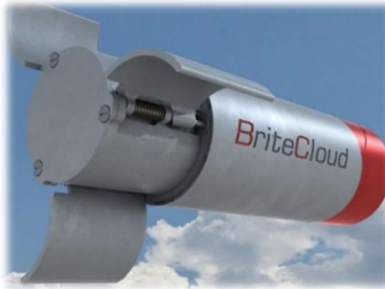
Figur 4.11: BriteCloud Expendable Active Decoy, November 2013 (illustration: Selex ES, CC BY-SA 2.0, via Wikipedia).
