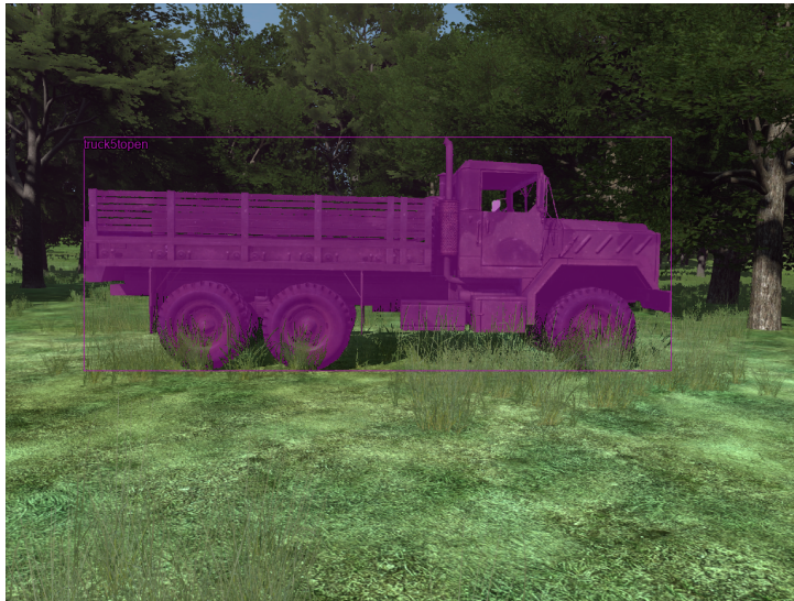
Figure 4.4: Synthetic image of a military truck, including its bounding box and segmentation annotation.
