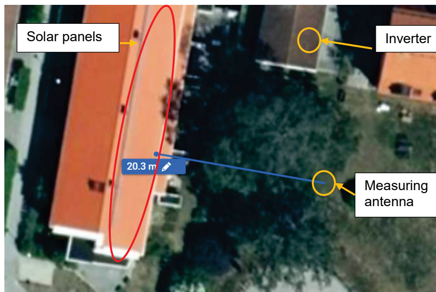
Figure 37. About 20 meters between the solar panels and the measurement antenna.
