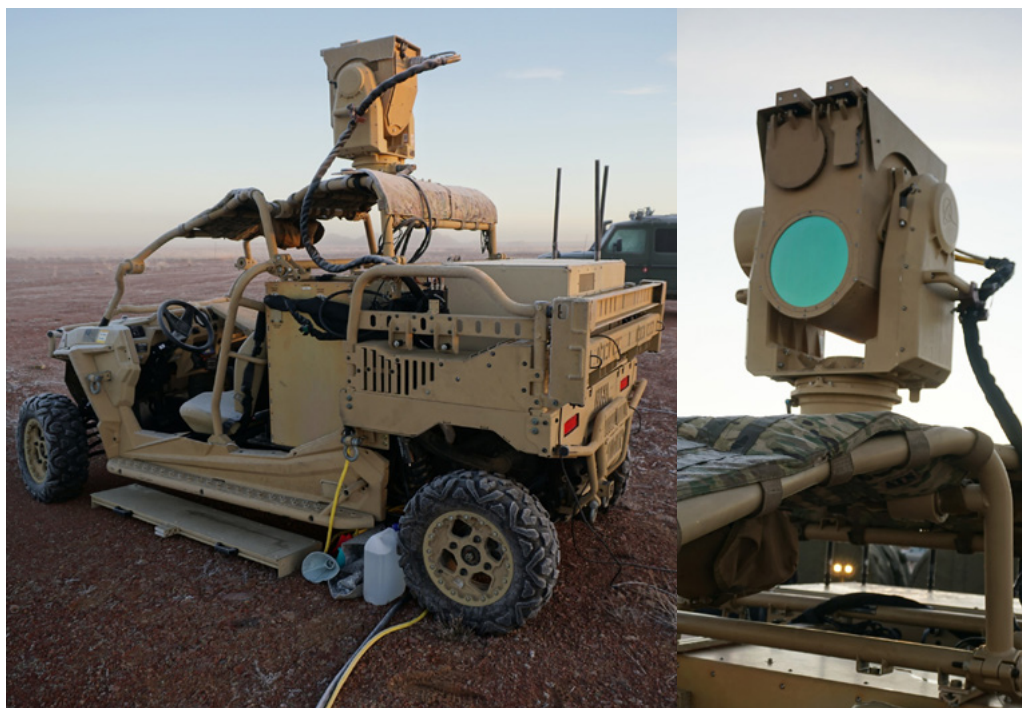
Figur 88. Fordonsburet laservapen CLWS (Compact Laser Weapon System).
