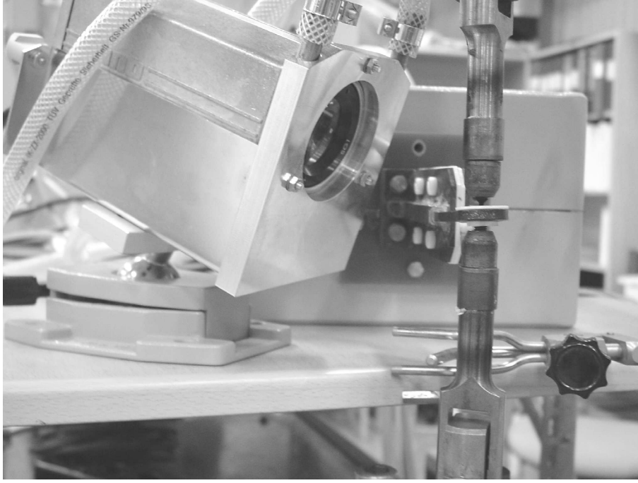
Figure 3. Close-up of the inductive heater and the IR-camera.
